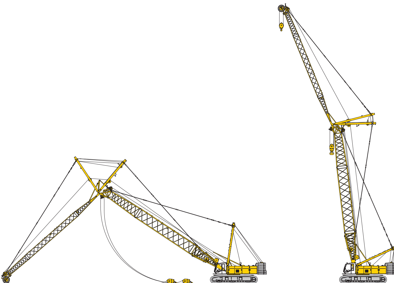
Erecting of main boom and luffing jib
